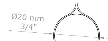
Detail 1:1 round hembar 3/4" (Ø20mm)
